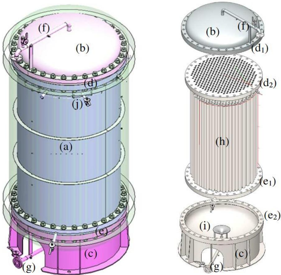
Schematic of a shell-and-tube Latent Heat TES (Bentivoglio et al, 2021, hal-03492919)
