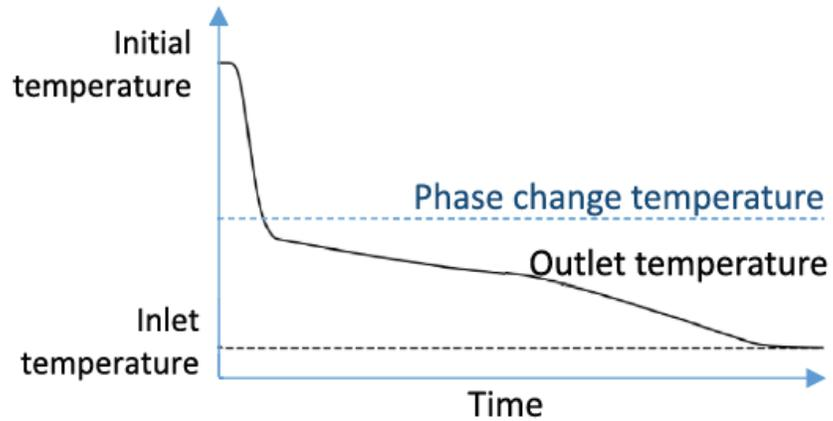
*Typical evolution of Latent Heat TES outlet temperature during discharge*
